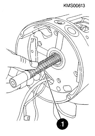
ASSEMBLING STARTING-MOTOR SOLENOID WITH CONTROL RELAY
